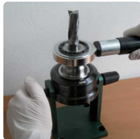
Tighten the nut using the torque wrench Art Z052 page 10.13
